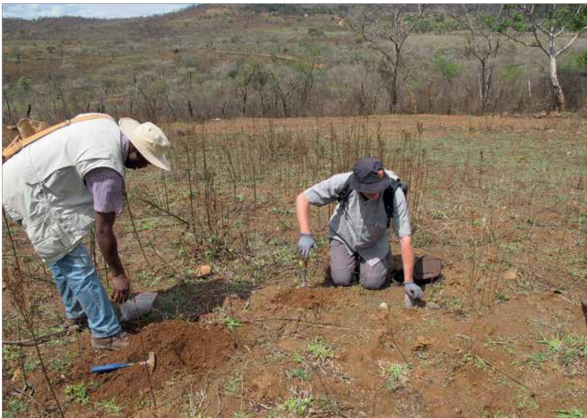
Fig. 5.2.17: Soil sampling in the centre of the eastern part of the Schiel Complex (Lombard's exploration camp from the 1930s). The apatite mineralisation does not crop out at all (Photo BGR).
